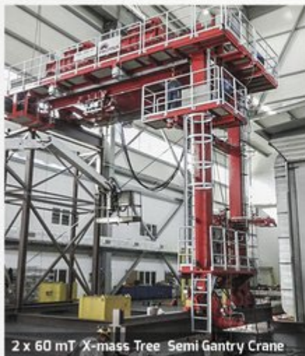
2 x 60 mT X-mass Tree Semi Gantry Crane
