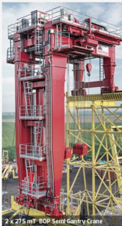
2 x 275 mT BOP Semi Gantry Crane
